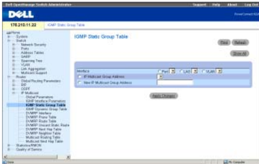
Figure 8-21. IGMP Static Group Table
