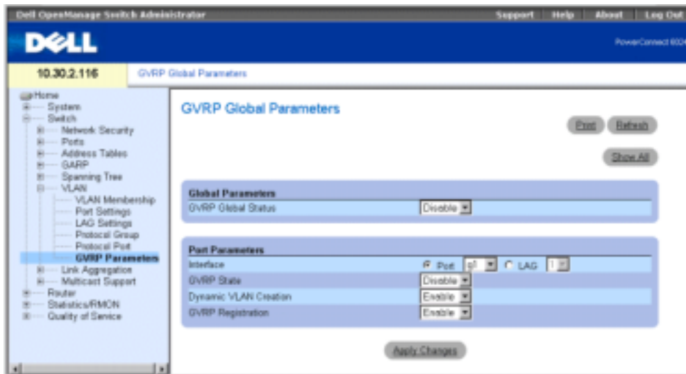
Figure 7-33. GVRP Global Parameters Page
